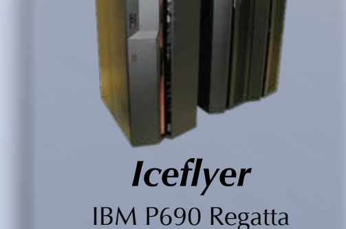
Iceflyer IBM P690 Regatta 32 Power 4 CPU 166.4 GFLOPS 64 GB RAM
