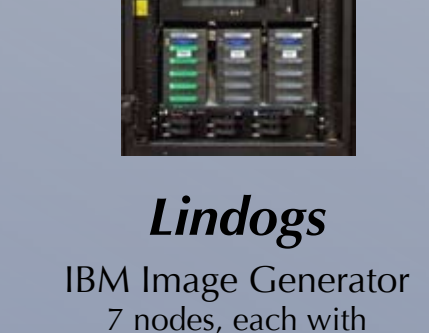
Lindogs IBM Image Generator 7 nodes, each with 2 Xeon processors at 3.06 Ghz 4 GB RAM 145 GB local disk
