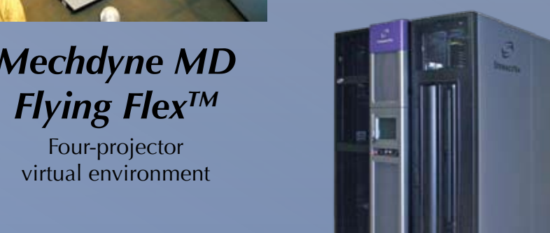
StorageTek SL8500 3+ PB Robotic Tape Library
