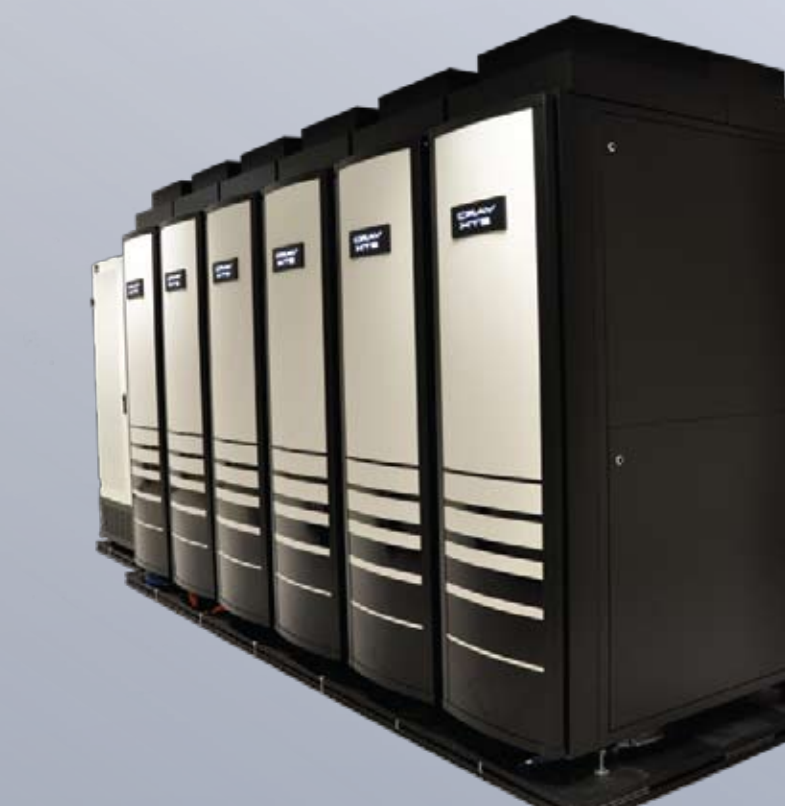
Pingo Cray XT5 3,456 compute cores 150 TB Lustre file system
