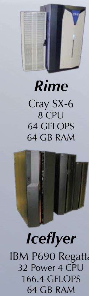
Iceflyer IBM P690 Regatta 32 Power 4 CPU 166.4 GFLOPS 64 GB RAM
